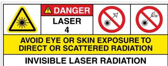
This label indicates the class of the combiner as a laser source, and warns about the potential hazards in case of exposure to the radiation.
