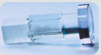
A highly transparent compound, deposited on chemically activated end-faces of two crystals, creates a bond that is extremely robust over time, temperature variations, and insensitive to mechanical vibrations. Dielectric mirrors coated at the end-faces of the crystals complete the monolithic assembly with no moving parts.
